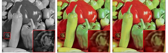
Fig. 1: Left to right: Bayer image, image reconstructed using OMP, and image reconstructed using the proposed method. While OMP takes 16 minutes, the proposed method takes only 1.5 minutes with little or no loss in reconstruction quality.
