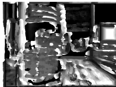
Figure 6.6: Bad depth map. While the depth calculation at the edges is expected to be accurate, the obtained depth map has erroneous edge values.
