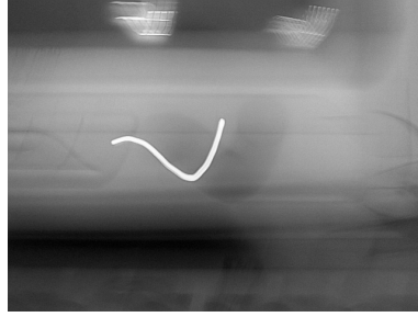
Figure 4.3: Actual image showing the point spread function, which acts as our ground truth measurement.
